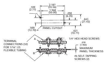
The Connector joins up to 32 tubes of  $\frac{1}{16}$ " I.D. tubing. The connector is joined together by two hex head screws and can be panel mounted.
