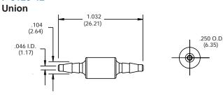
Barbed ports for  $\frac{1}{10}$  I.D. flexible tubing. Material: Polysulfone
