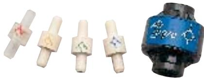
The F-2804 Series Check Valves permit flow in one direction only. The operation of the check valve is based on the movement of a small disc. The disc shifts within the housing as the pressure differential changes from forward to reverse. A flat surface on one side of the disc seals off flow, while the other side allows flow to pass.
