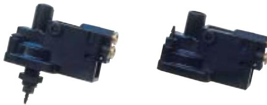
The V-5700, V-5800 Series Vacuum Piloted 3-Way Valve has an adjustable vacuum pilot setpoint. The adjustable vacuum pilot can be set to sense vacuum between 1 to 28" Hg. Maximum vacuum of 29.9" Hg. The 3-Way Valve is Normally Open or Normally Closed. The Normally Open valve senses the adjusted vacuum setpoint and turns the output off. The Normally Closed valve senses the adjusted vacuum setpoint and turns the output on.
